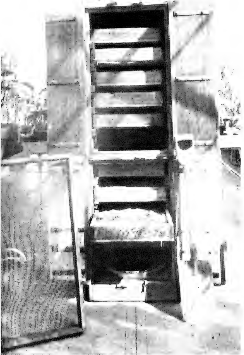
FIG. 57.—Home-made device for steaming infected soil. It is a steam-chamber holding 12 drawers having wire-mesh bottoms. These slide in and out on rollers.
